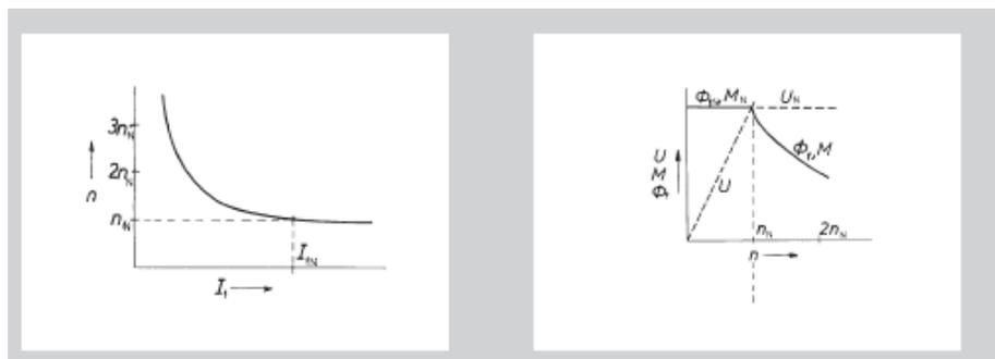
Operating diagram of a speed-variable DC motor
