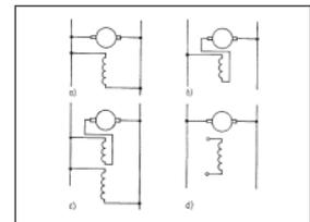
Exciter winding circuit for DC machines
