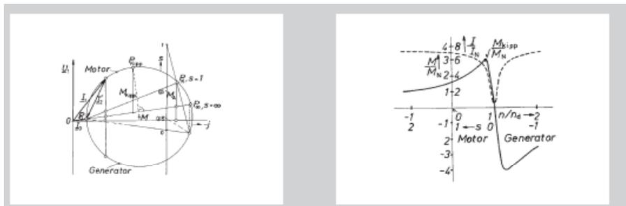
Diagram of the stator current
