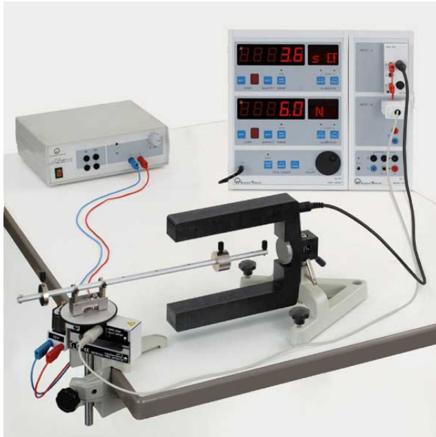
Centrifugal force on a revolving body – measuring with the central force apparatus and CASSY (P1.4.3.3)
