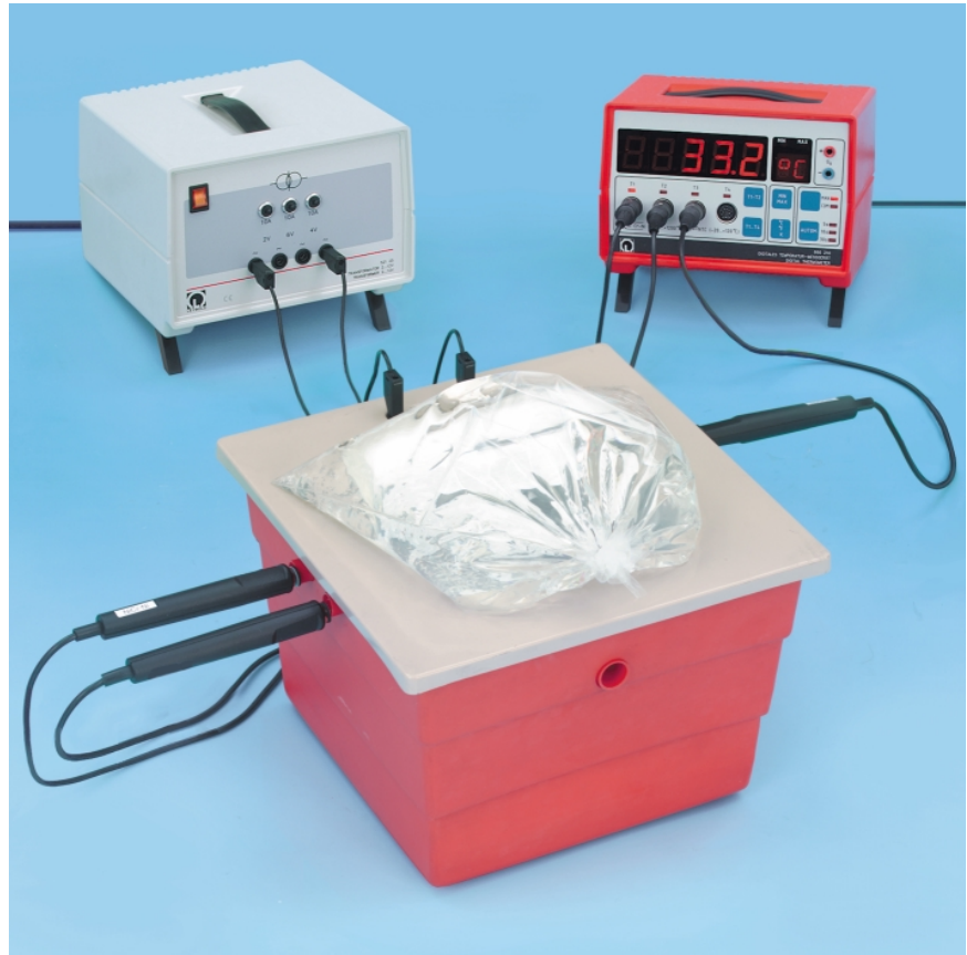
Determining the heat conductivity of building materials with the aid of a reference material of known thermal conductivity (P 2.2.1.2)
