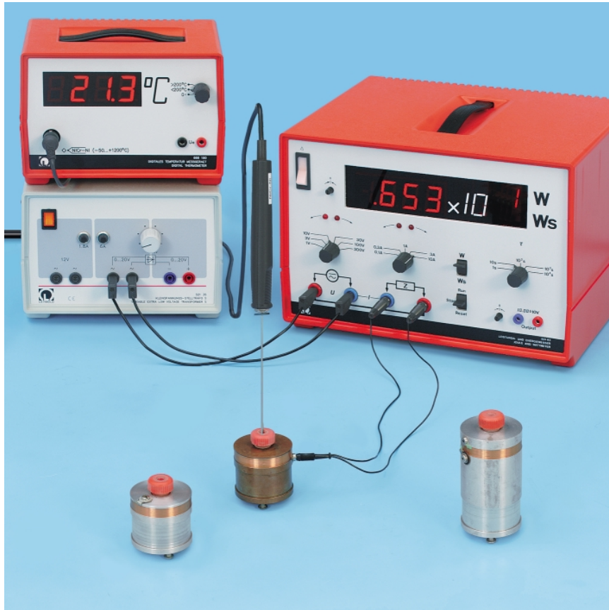
Converting electrical into heat energy - measuring with the joule and wattmeter (P 2.3.4.2)
