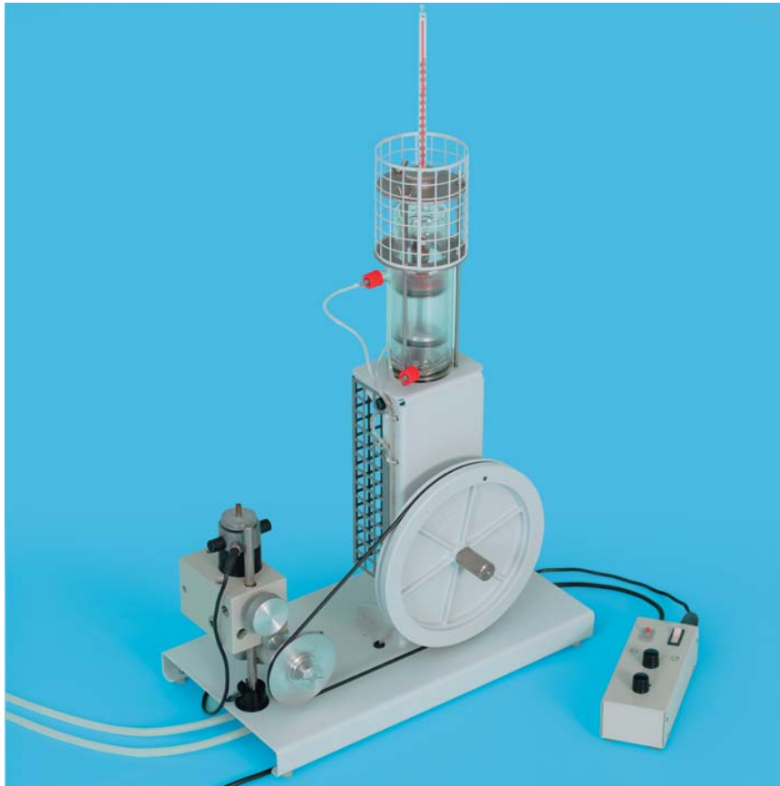
Operating the hot-air engine as a heat pump and a refrigerating machine (P 2.6.1.3)
