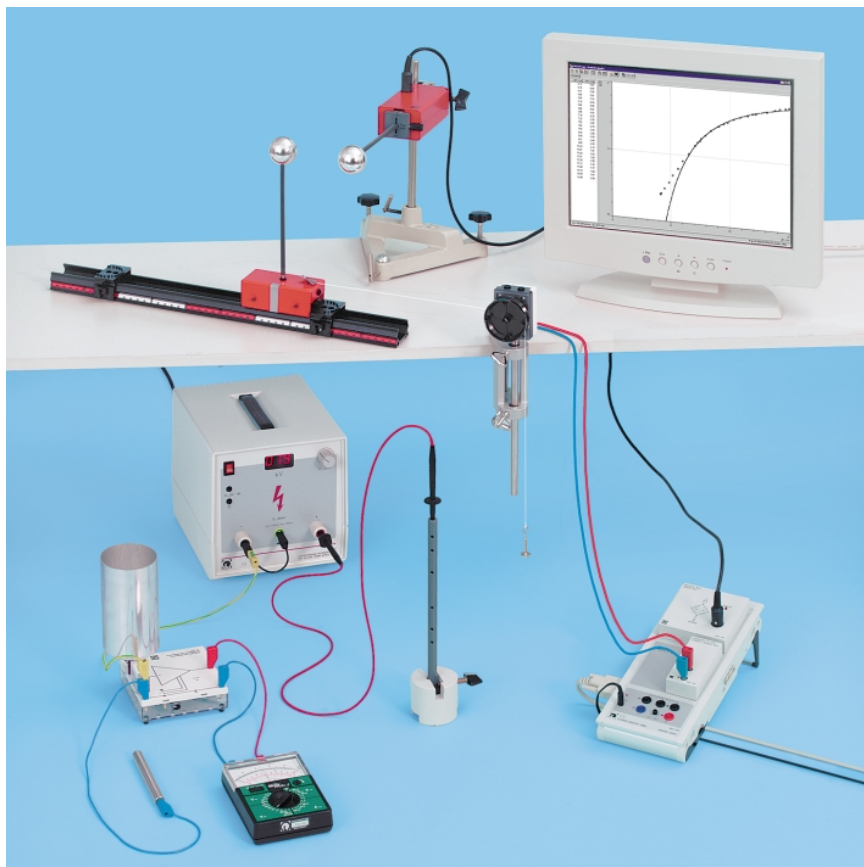
Confirming Coulomb's law with displacement sensor and CASSY (P 3.1.2.3) (old equipment)
