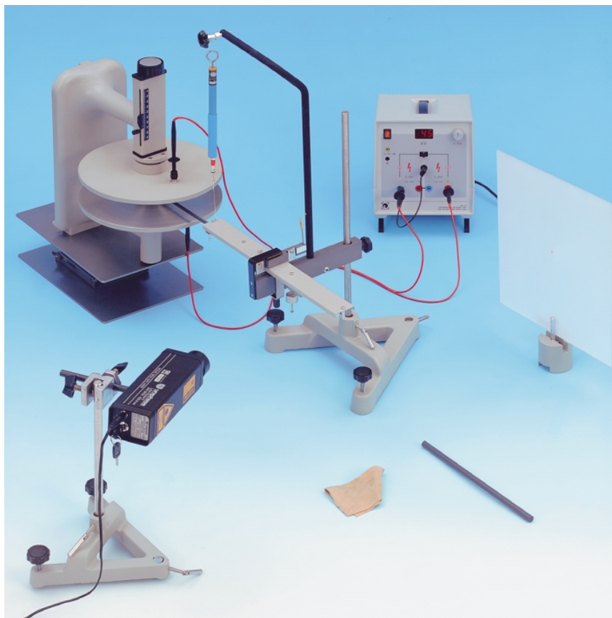
Measuring the force of an electric charge in a homogeneous electric field (P 3.1.4.1)
