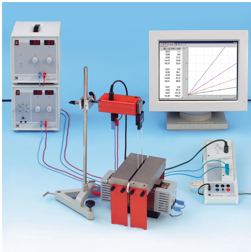
Measuring the force acting on current-carrying conductors in a homogeneous magnetic field – Recording with CASSY (P 3.3.3.2)
