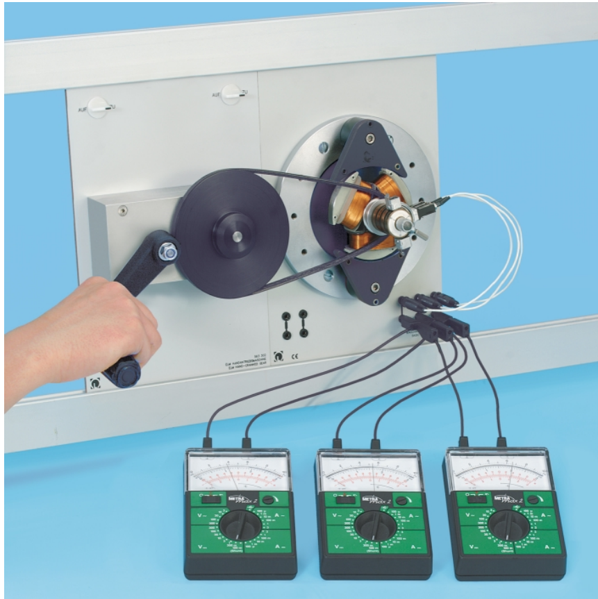
Experiments with a three-phase revolving-armature generator (P 3.5.4.1)
