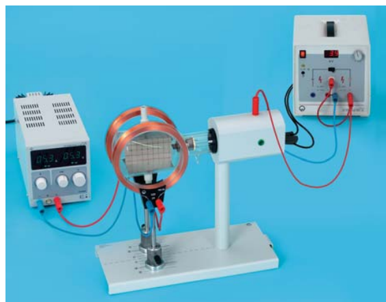
Investigating the deflection of electrons in magnetic fields
