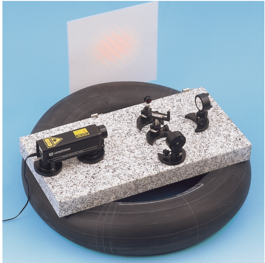
Setting up a Michelson interferometer on the laser optics base plate (P 5.3.4.1)
