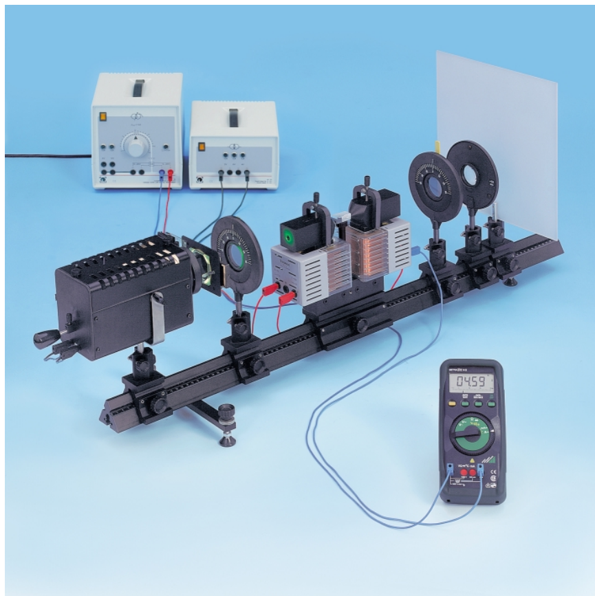
Faraday effect: determining Verdet's constant for flint glass as a function of the wavelength (P 5.4.6.1)
